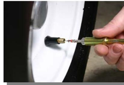
Position the valve stem between the 4 and 8 O'clock position and remove the valve stem. The tire will deflate. (fig. 1)
