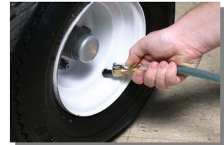
Attach the brass connector from Arnco's ReSeal pump to the valve stem (fig. 2)
