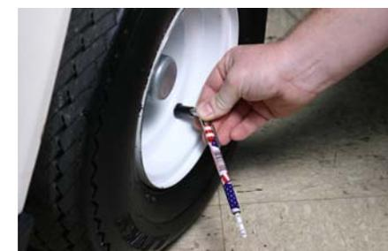
Inflate tire and check for proper operating pressure. (fig. 4)
