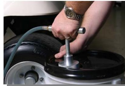
Pull up on the handle and inject the proper amount of ReSeal into the tire. Each stroke delivers 6 ounces. (fig. 3)
